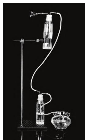
Fig. 5 Oxygen supply device based on siphon principle
