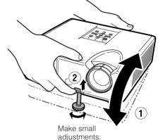
3 Use the rear adjustment foot to make the projector level.
